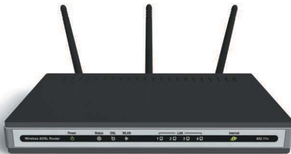
Figure 8-13 802.11n access point with three antennas
