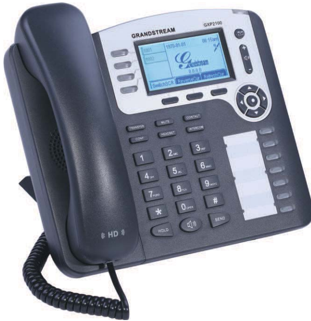
Figure 12-6 An IP phone Courtesy of Grandstream Networks, Inc.
