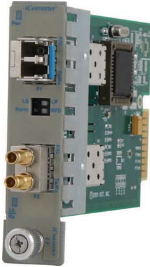
Figure 3-39 Fiber to coax converter
