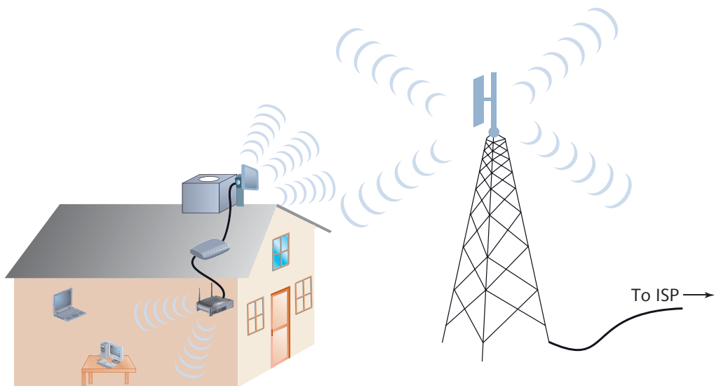
Figure 8-21 WiMAX service provider's antenna
